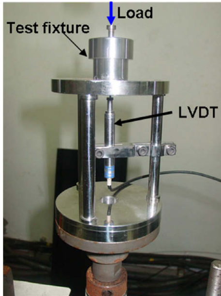
Fig. 4. The experimental setup of shear punch tests showing the LVDT attachment coupled to the bottom of the specimen clamped in the test fixture.
