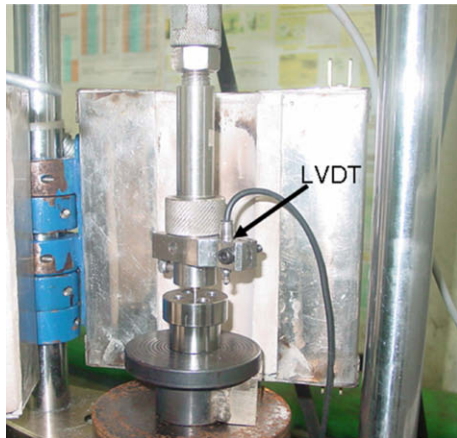
Fig. 5. The experimental setup where LVDT is coupled to moving punch for measuring the displacements.
